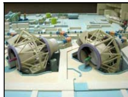
3-D models of two gantries realized on ISAT Hall's Rapid Prototyping Printer.
