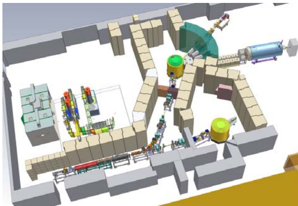
Fig. 1 Schematic layout of the LENS facility showing the accelerator and RF power systems on the left, the radiography/irradiation target station on the lower right, and the cold neutron target station and its associated instruments in the upper right.
