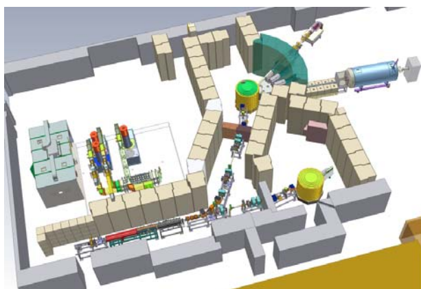
Fig. 1 Schematic layout of the LENS facility showing the accelerator and RF power systems on the left, the radiography/irradiation target station on the lower right, and the cold neutron target station and its associated instruments in the upper right.
