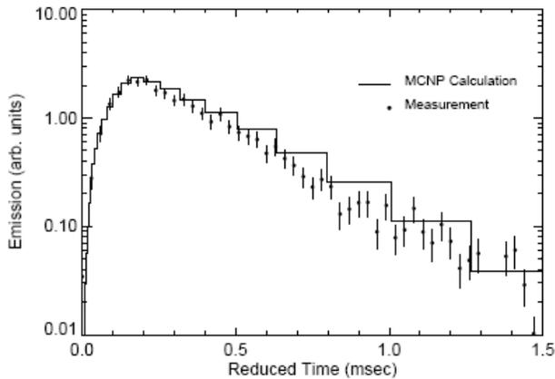
Figure 3 Emission time distribution for neutrons with energy 2.74meV measured for a moderator temperature of 4K, compared to MCNP simulations using the smeth22K kernel.
