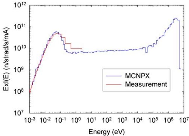
Fig. 4. Comparison of the thermal neutron spectrum with that predicted from an MCNPX calculation. The measurement was made with a <sup>3</sup>He detector positioned 5.7m from the target and normalized to an activation foil measurement
