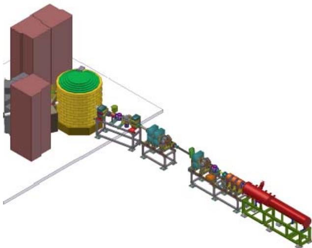
Fig. 1. Overall schematic layout. Shown are the accelerator (right-hand of the picture), the beamline and the TMR (vertical cylinder).
