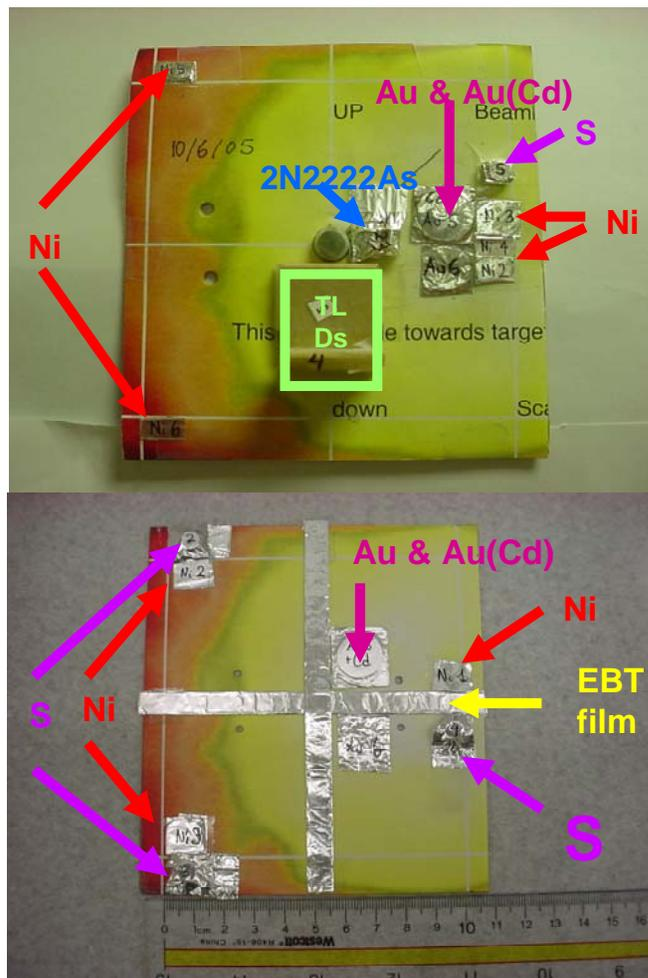
Fig. 2. Location of foils for two irradiations. The colored background is a position dependent MCNPX calculation folded with the <sup>58</sup>Ni(n,p)<sup>58</sup>Co cross section. For details see text.
