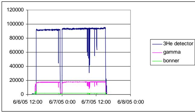
Fig. 3. Monitor detector rates during a 24h irradiation. The gamma detector and the bonner sphere monitor the room background, while the <sup>3</sup>He detector monitors the thermal flux from the target.
