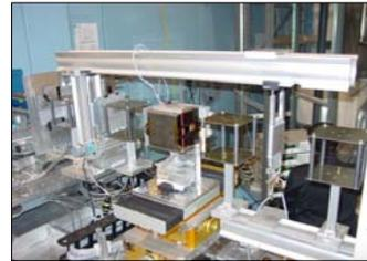
The solenoid pair was energized with 5 Amps, giving an internal field of ~45Gauss. Single spin-state intensity was measured as the solenoid pair was translated across a 50 micron-wide beam. This was repeated for 4 angles (see image left, results below). The frequency of the intensity vs. displacement remained constant as the triangle pair was translated.
