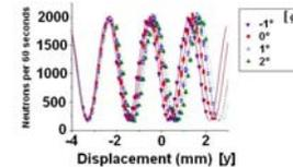
The intersection of the intensity curves for the 4 angles indicates the location of the physical center of the triangle pair (~-4mm in above figure). The results of the experiment
