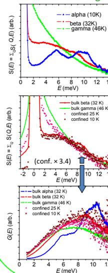
The generalized density of vibrational states,  $G(Q, E)$ , is calculated from the one phonon scattering function,  $S(Q, E)$ , using:
