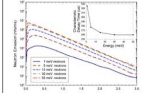
Simulated Emission Time Distribution from 22K Methane Moderator. For  $E > 5$  meV pulse shape is dominated by the  $\text{H}_2\text{O}$  reflector
