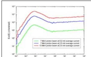
Simulated Optimal Neutron Spectrum from 22K Methane Moderator at different stages of accelerator development
