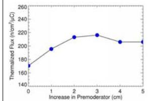
Simulation of improvements in premoderator in constructed geometry. A 3-4 cm thick layer of hydrogenous premoderator material placed in the vacuum gap between the target and moderator should enhance the thermalized flux coupling to the cold source by 25%.
