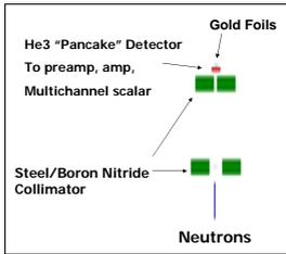
We simulate the ToF spectroscopy experiment at 5.7 m, 20 degrees to the moderator normal in MCNP for a 22K methane moderator.
