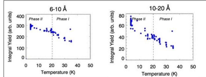
Cooling the moderator increases the long wavelength neutron flux considerably. However, the phase I-II transition in methane (indicated by dashed line) appears to be influencing the 6-10 Angstrom behavior.
