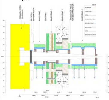
Fig. 2: Schematic of collimators and primary shielding for SANS PFP.
