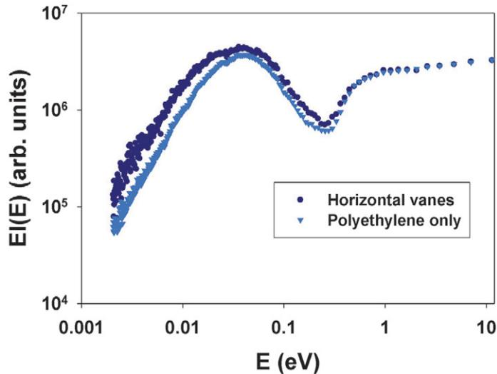
Fig. 2 Lethargy flux measured from two moderators inserted into the LENS TMR and held at a temperature of 60K. One is a laminated composite of polyethylene sheets and horizontally oriented single crystal vanes of Si, and the other is a simple stack of polyethylene sheets. We note that the intensity from the composite moderator is approximately a factor of 2.5 greater at energies on the order of a few meV.
