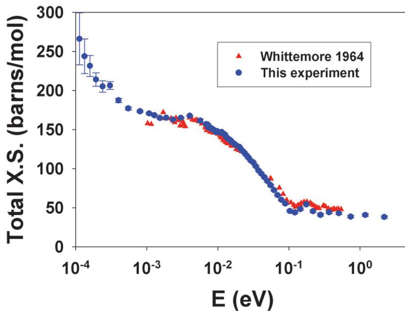
Fig. 1 Total cross section of ZrH<sub>2</sub> as measured on the SANS instrument at LENS demonstrating our ability to reach energies on the order of 0.1meV in such measurements. Data collected at LENS are compared with data published in [6].
