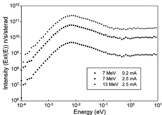
Fig. 1. Monte Carlo simulations of the neutron intensity for the proposed LENS facility operated with a Be target at three different power levels. The lowest power level shown gives the anticipated flux in phase I of the facility, the second the flux after upgrading to 50 mA and 5% duty factor at 7 MeV, and the last at the facility's ultimate power of 13 MeV, 50 mA and 5% duty factor.
