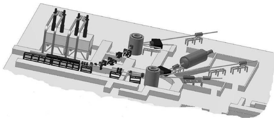
Fig. 2. Schematic layout of the LENS cold neutron facility. Showing the accelerator with its associated RF power systems on the left, one target station for neutron scattering with three instruments (to the right), and a second target station for conducting research into neutron radiation effects (upper left).
