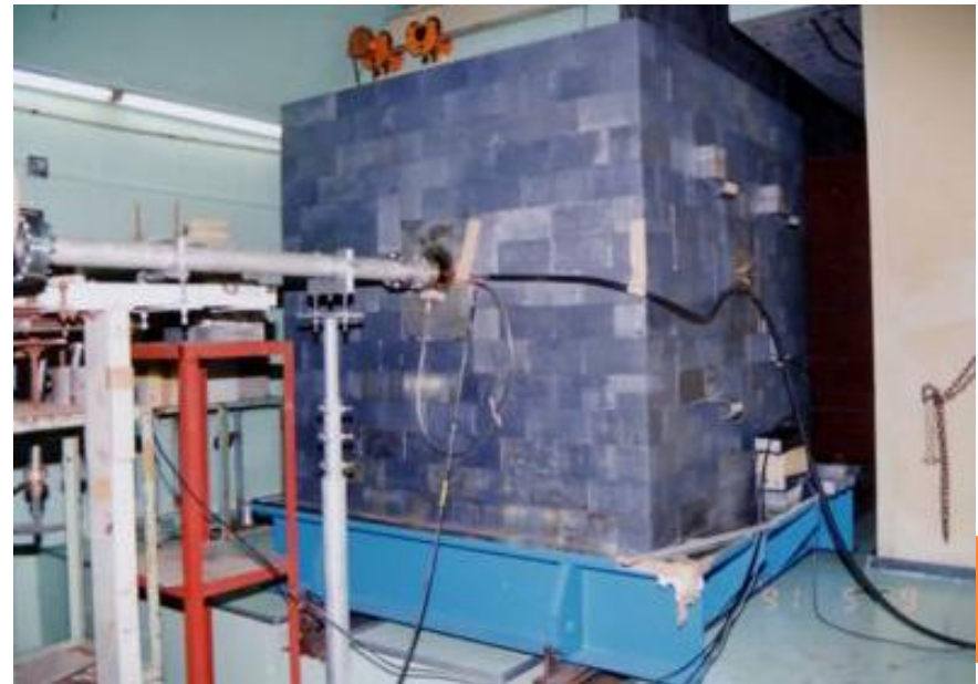
Lead spectrometer ( 1.5 \times 1.5 \times 1.5 \text{m}^3 )
