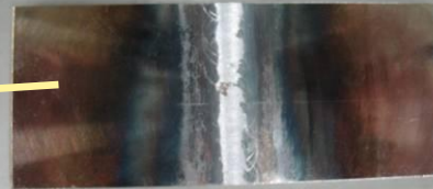
Fe-Fe welded sample
