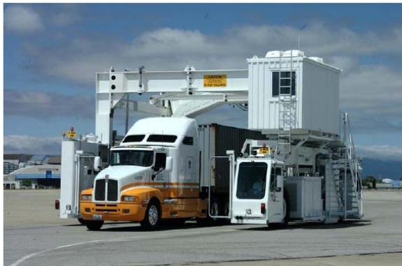
Figure 5. Aracor Eagle® relocatable x-ray inspection system inspecting a fully loaded truck.
