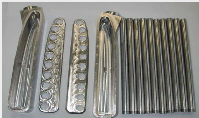
2. Zr cooling system manifold & collector plates
