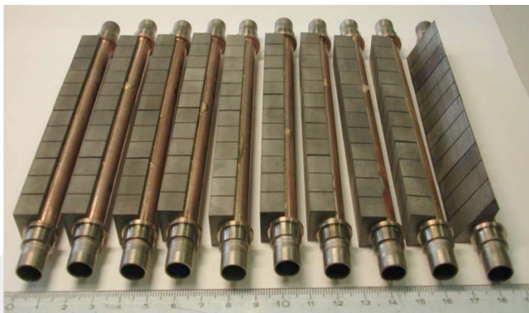
1. Be-tile brazed cooling pipes with Zr adapters
