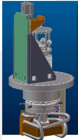
Fast Emittance Scanner (FES): high resolution q - q' rms emittance in less than 2 seconds
