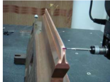
Three-coordinates measurement (Platform size: 800mm × 1.4m)
