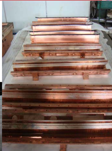
6 horizontal electrodes after fine-machining
