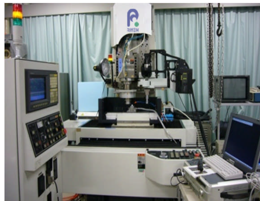
3D internal structure microscopy (Slicer)
